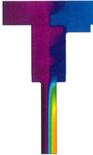
Figure 7: Top rail and header with door stop and weather stripping and edge of glass thermal profiles
